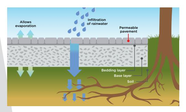
The pavers used in a permeable installation are made with extra space between them so rainwater can flow through permeable base materials and back into the earth below.
