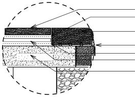
Unilock Natural Stone paving units 7/8" (22mm) thick Bond/Slurry coat must be applied to back of flagstone
