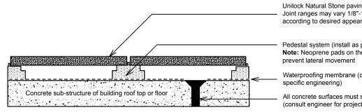
Unilock Natural Stone paving units 7/8" (22mm) thick Joint ranges may vary 1/8"-1/4" (2.5mm - 6.4mm) according to desired appearance
