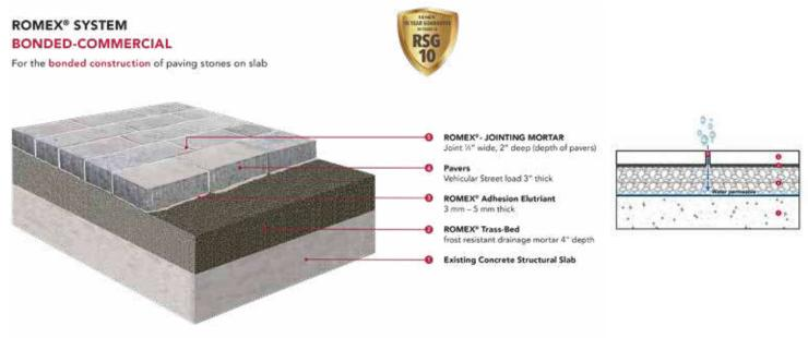
Ideal for garage access, parking spaces, etc. Vehicle traffic up to 40 tons is permitted for occasional use (delivery trucks, emergency vehicles, etc.) Minimum requirement for fastenings/surface covering: Minimim nominal thickness = 75mm (3")
