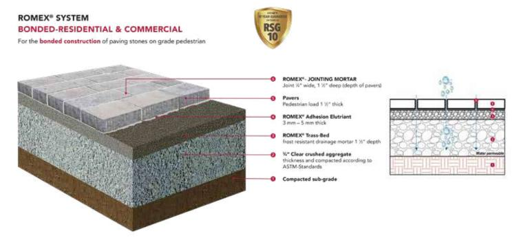
Minimum requirement for fastenings/surface covering: minimum nominal thickness = 50 - 100mm (2-4")
