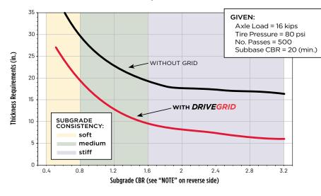
Aggregate thickness is based on Giroud-Han design methodology for unpaved roadways, using 1.5 inch maximum rut depth. Any ruts that occur prior to paver installation should be filled with additional aggregate or bedding material. Additional aggregate will be required if traffic loading or passes will exceed those given above prior to paver installation.
