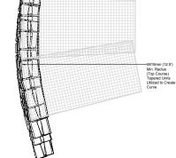
Geogrids will overlap and should have 75mm of compacted soil between the layers. (Geogrids should be spaced on blocks so overlap does not occur until geogrid enters soil zone as shown)
