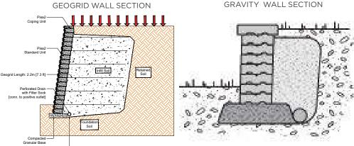
Cross sections are examples, and must not be used for construction.
