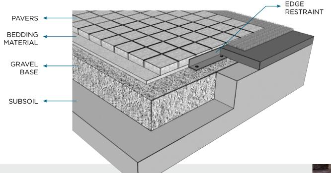
A proper base will ensure that your pavers and walls won't settle or shift out of place with freeze-thaw cycles.
